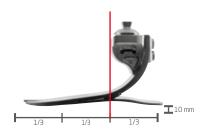
Divide the sagittal plane of the foot into three thirds. The alignment reference line should run through the centerpoint between the two posterior thirds. The alignment reference line is different for each of the three feet.
